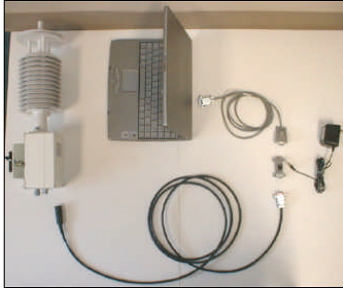
Figure 12. MET to PC Connection
