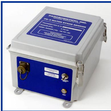
PS-2 Enclosure Kits are designed to accept Series 1000 Intelligent Transmitters with RS-232 interface. The enclosure kit is comprised of a splash-proof box, over-pressure relief valve, wiring harness and connection hardware.
